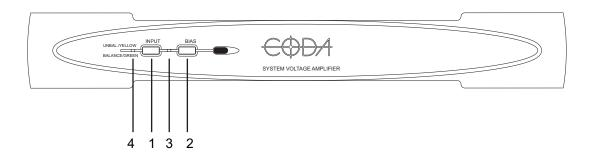
Note: If a power interruption occurs to the system, immediately turn the BIAS power OFF on the front of the SV. The resumption of power will cause no noise pulses in the Amplifier System S150/250. However, some sources may produce high output voltages on turn on, which may cause damage to the amplifier or speakers.
