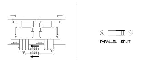
The OPERATION SELECTOR is now commoning the inputs of the S150/250, so the cable from the SV may plug into either LEFT/CH A or RIGHT/CH B. This configuration is used for bi-wiring or driving two sets of speakers, were total isolation of speaker components is required. The amount of power from each of the four output channels is 100 Watts class A (S150).
