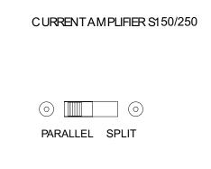
The OPERATION SELECTOR is now commoning both channels of the inputs and both channels of the outputs of the S150/250. The cable from the SV may plug into either LEFT/ CH A or RIGHT/CH B input and the speaker leads may be attached to either LEFT/CH A OUTPUT or RIGHT/CH B OUTPUT. The amount of power from each channel is 100 Watts class A (S150), however, since there are two output stages in parallel, current capability is doubled insuring pure class A power into 4 Ohms of 200 Watts .
